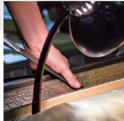
Hand scraped double V table ways
