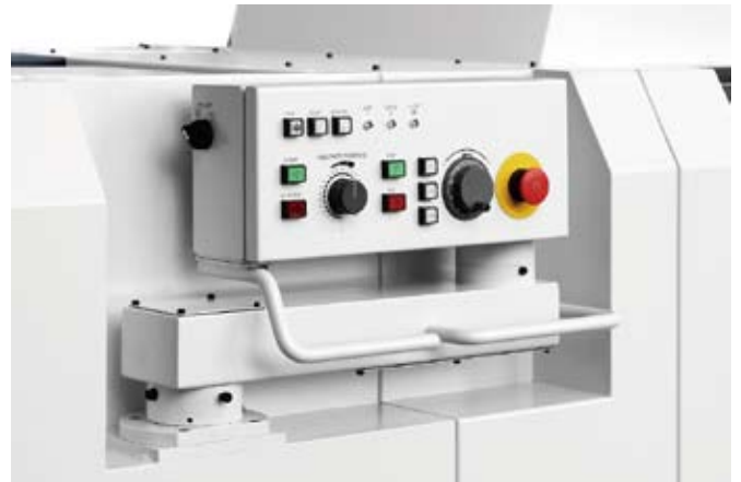
Sub operation panel
