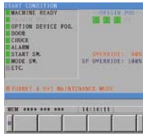
START CONDITION Used to set the start conditions for automatic running.
