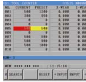
TOOL COUNTER Used to set and reset the tool counter stop value and enter the tool wear offsets.
