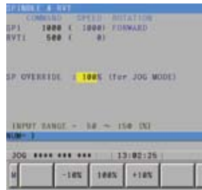
SPINDLE & RVT Used to set the rotational speed of the spindle and revolving tools. Used to set the spindle override.
